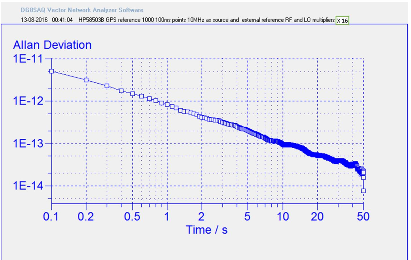
The Allan deviation demonstrates a slightly better system performance with the HP58053B, e.g.  $9 \times 10^{-13}$  against  $1 \times 10^{-12}$  at 1 sec measuring time for the Leobodnar GPSDO. This is mainly due to the rise time for the external reference square wave is faster for the HP58503B setup as a homemade shaping device used.
