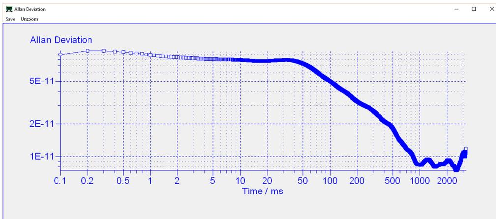
Below measurements made for 10000 100mS points at 500MHz average stability calculated to 4.03E-11
