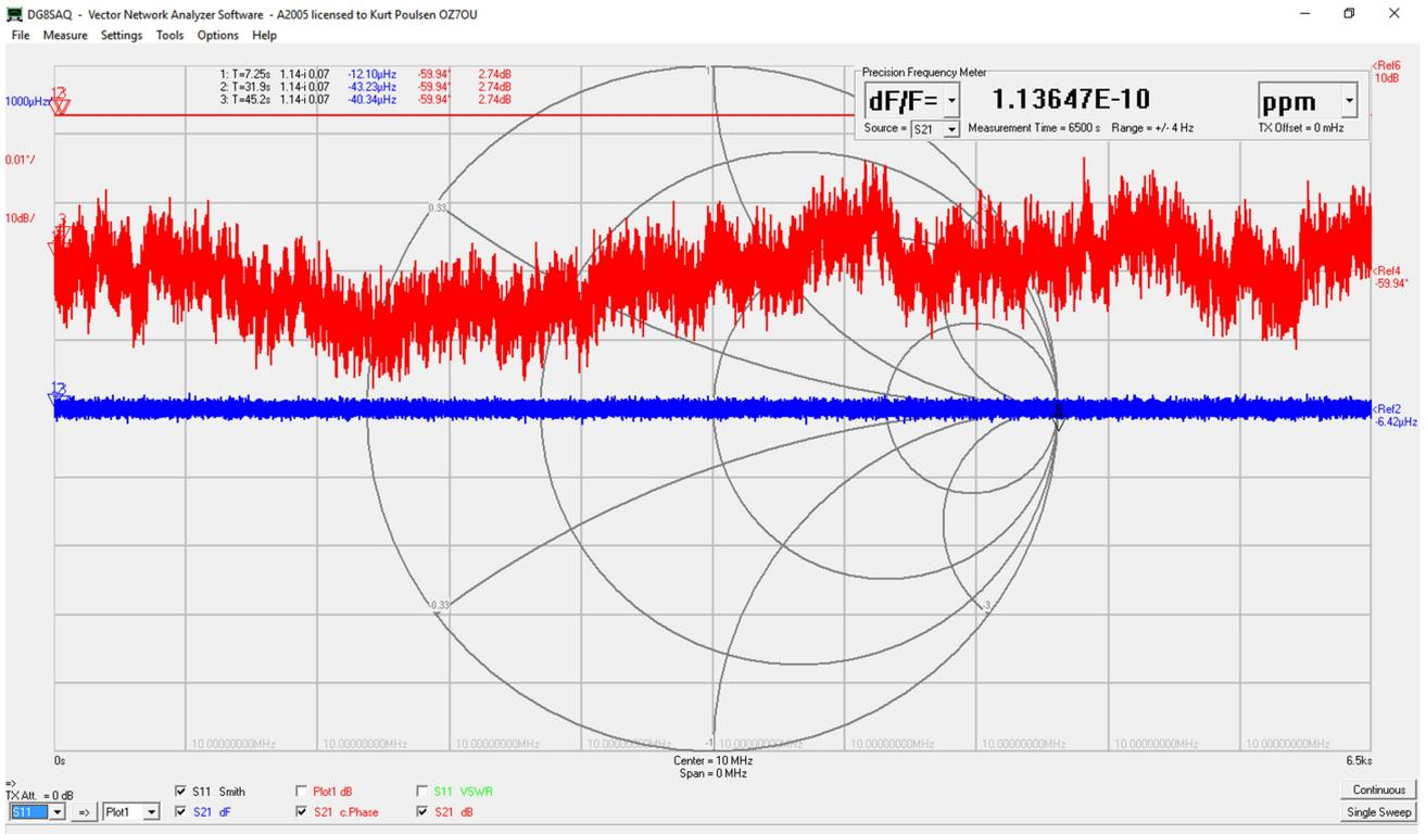
Leobodnar sweep for 65000 100ms points both as external reference at 13.3dBm and signal source to RX port of -16.7dBm. The External reference input is High Z so a SMA T adaptor used for signal distribution
