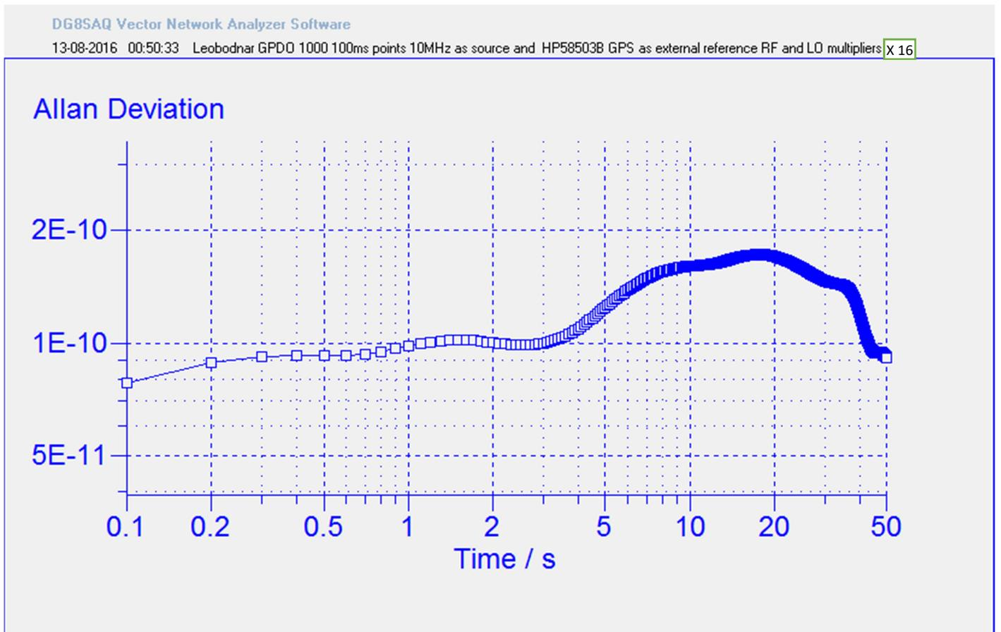
The Allan Deviation does not follow the usual trend for an oscillator due to the design principles of the circuitry. It has however an excellent short term stability maintained over time. It will be seen later on that the Leobodnar GPSDO is very fast to reach this stability, thus a perfect tool for field usage as spot on very quickly. See However next measurements with 65000 points
