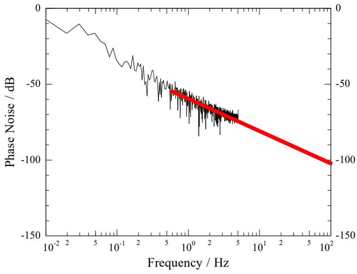
1000 100mS points at 11.9MHz and if a linear curve it will hit about -100dB
