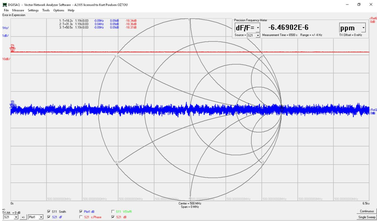
Leobodnar GPSDO measured for 65000 100ms points against the HP 58503B GPS disciplined 10MHz reference. Use of the outdoor marine GPS antenna has caused a more stable trace with less ripple compared to the previous measurement made with the supplied small magnet antenna also placed outdoor, but not with complete 360 degree view.
