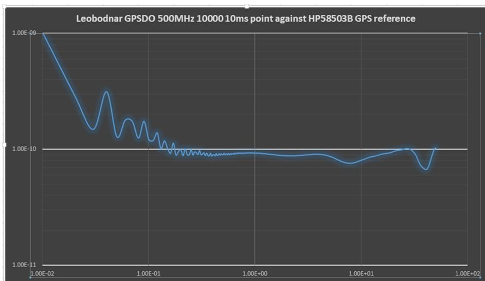
Allan Deviation for 10000 10mS points at 500MHz and same result as before with slightly more stable frequency due to outdoor marine GPS antenna
